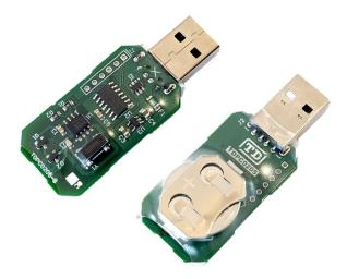
The "Clock Dongle" is a Real-Time Clock (RTC) used to obtain the current date and time. It is designed to be used in conjunction with computers that lack battery backup, such as single-board computers. Even without computer power, it can continuously provide the current time. It is compatible with both Windows and Linux.
